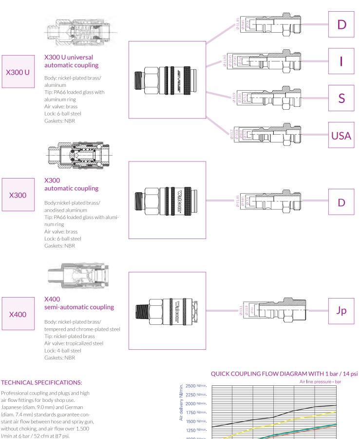
Operating air pressure: 0 - 16 bar / 0 - 232 psi Working temperature: -40°C + 80°C
